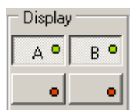
Fig. 5.4.1. – Channel visibility controls
