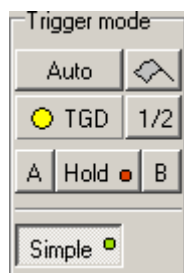
Fig. 4.1.8.2. – Trigger mode controls with separate hold controls
